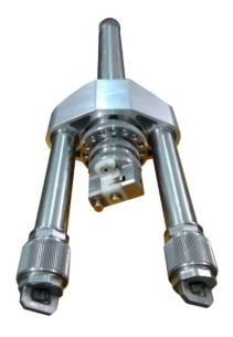
EAD-20S breech has a safety pin to keep the terminals short and cartridge is connected just when it has been deployed. This enables a bomb technician to set up the disruptor at the incident control point and spending minimum time at IED
