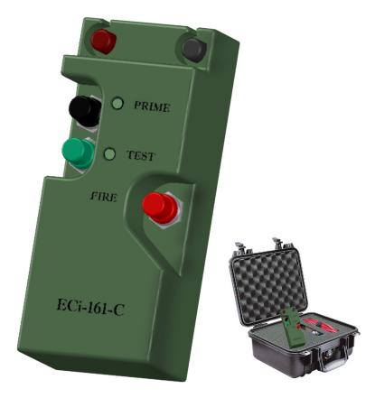
Single circuit Electronic Exploder; is a light weight two hands fire system. It provides the same reliably of four circuit Shrike. It can check the continuity of firing circuit. The unit is primed before fire and the firing is done by simultaneous pressing of the fire and prime buttons. The firing circuit remains inhibited till the system is not fully primed.
