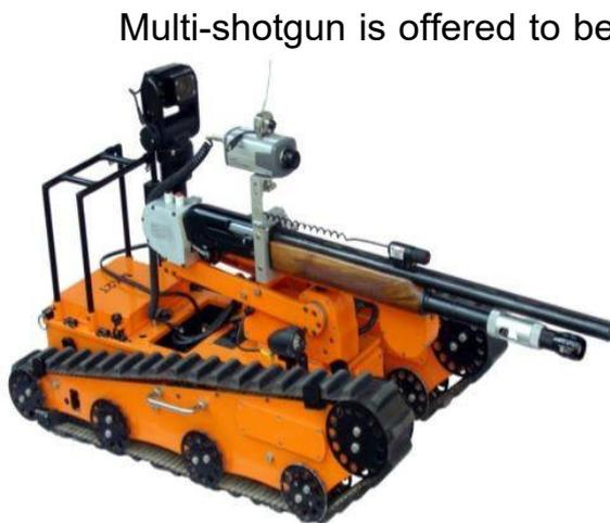
Multi-shotgun is offered to be mounted on a frame incorporating the Firing Actuation Mechanism, Laser Aiming, Camera and LED light. In EOD or IEDD operations remote controlled shot guns are used to gain access or shoot an area of interest. The gun used for the system is a multi-shot and semi-automatic. The gun has the capability to fire five shots. To install the gun on any robot the complete assembly is fitted to the Arm of the robot and connected to the local firing terminals.
