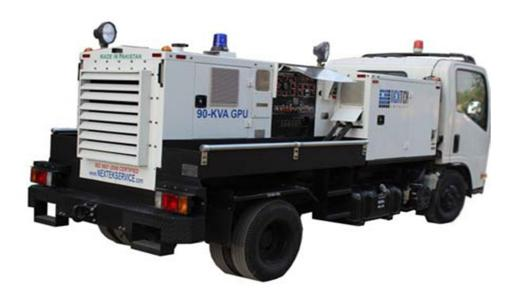
90KVA Ground Power Unit (GPU) is a reliable Mobile Power Source for the aircraft startup and its maintenance activities. It employs Marathon Alternator and Cummins engine. The system can be customized as trolley mounted or a vehicle mounted. The system employs various safeties and protections to be used with the military aircraft. The GPU has been developed on Aerospace and military standards and has underwent a rigorous qualification program.
