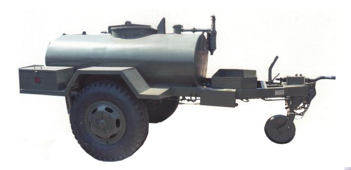
This 400 gallon Water trailer is a  $1\frac{1}{2}$  Ton, 2 Wheeled and offered in Stainless steel or Fiberglass tank body. These Trailers also referred to as Water Buffalo are designed to carry potable or non-potable water either highway or cross-country routes. It can be towed by a  $2\frac{1}{2}$  Ton Truck or equal with allowable speeds of 80 km/h highway and 48 km/h cross-country.
