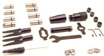
Fuze projector or a De-armer deal with the fuzes of UXOs for breaking its detonation train. De-armer has specially designed barrel, with slugs to be fired by a cartridge. De-armers disrupts fuses with cocked strikers. Electric 0.5" cartridges or de-bulleted 0.5 " rounds are used in it. A fork can be used for a lower velocity attack on some specific fuses. This tool can also used against Improvised Explosive Devices (IED's) also with special shot load.
