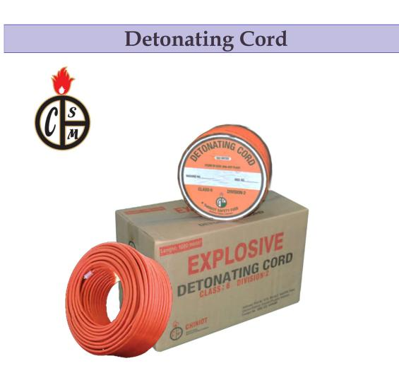
Detonating cord consists of PETN core covered by woven tube of polythene tape and cotton threads protected by an outer PVC insulation. The weight of cord is approximately 10 g/m and outer diameter is about 5.0 - 5.5mm. The Cord is a strong, Flexible and linear explosive. It is cap sensitive product having the ability to initiate all cap sensitive explosives & primers.
