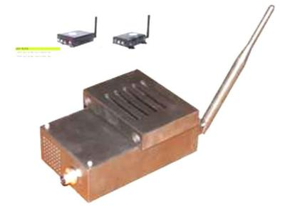
Various audio/ video sender's/ receivers options for EOD Robots facilitate aiming and robot tools' operations monitoring. The audio and video senders for EOD robots have been developed for monitoring the tools operations and for the aiming of the weapons to be fired.
