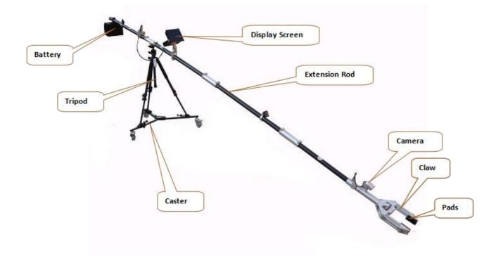
**PCM-03 IED Manipulator** provides an IED operator a stand of for 4 meters when already protected by an EOD suit. The claw's open and close is controlled through visual feedback as well as through a LCD screen. Situation of a safety distance of 3 meter or more has significant chances for an EOD operator's survivability with EOD Suits having overpressure suppression. Apart from moving suspect objects, the manipulator can be used to position disruptors, x-ray equipment and other EOD equipment.
