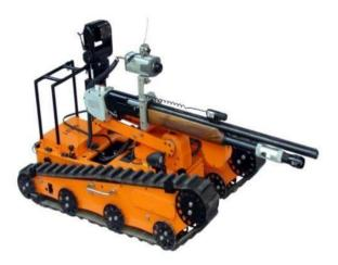
Multi-shotgun is offered to be mounted on a frame incorporating the Firing Actuation Mechanism, Laser Aiming, Camera and LED light. In EOD or IEDD operations remote controlled shot guns are used to gain access or shoot an area of interest. The gun used for the system is a multi-shot and semi-automatic. The gun has the capability to fire five shots. To install the gun on any robot the complete assembly is fitted to the Arm of the robot and connected to the local firing terminals.
