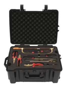
Nonmagnetic kits are essential for working in EOD/ IEDD tasks to avoid threat of magnetic field and spark initiating of an IED or a UXO. Tools are made of Beryllium-Bronze alloy (Be-Cu) king it 100% non-magnetic tool set but also it is a non-sparking tool kit. The kits are also suitable for safe working in other explosives atmospheres like a gas station, fuel Shops or where volatile fumes exist. All tools are suitable for contact usage and are supplied individually certified.
