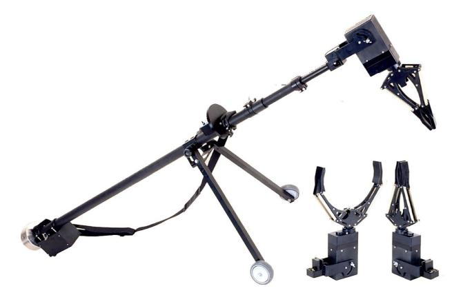
The PKM-02 UXO Manipulator is a lightweight telescopic arm designed to offer a 3-meter standoff distance when the operator is already protected by an EOD suit. The manipulator consists of three sections with locking mechanisms to securely hold the extended position. At the end of the telescopic arm is a universal mount for installation of different tools. A mechanical claw is the important tool installed. A counterweight and battery box are installed on the other end.
