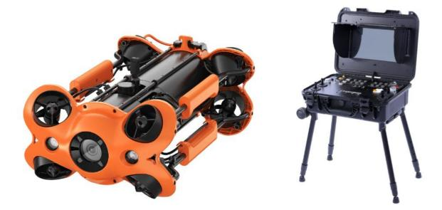
The HWM-2 is a specialized underwater remotely operated vehicle (ROV) for professional and industrial purposes. It is lightweight aluminum alloy with compact body weighing less than 6KG (13 lbs) for single person portability and quick deployment in 3 minutes. It features a configuration of 8 Vectored Thrusters, enabling seamless movement in all directions. The ROV utilizes a hybrid power system, combining AC and battery power, to achieve an unlimited battery life.
