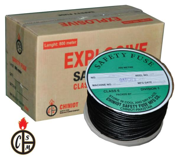
Safety Fuse is a flexible fuse cord with inner core containing special grade black powder and is covered with textile yarns. For water proofing, fuse is insulated with uniform PVC coating. Safety Fuse burns slowly for transmitting of the burn to a detonator providing time for the demolition team to evacuate from the area.
