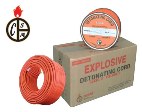
Detonating cord consists of PETN core covered by woven tube of polythene tape and cotton threads protected by an outer PVC insulation. The weight of standard cord is approximately 10 g/m with our diameter of 5.0 – 5.5mm. The Cord is a strong, is Flexible and has linear explosive. It is cap sensitive product having the ability to initiate all cap sensitive explosives & primers.
