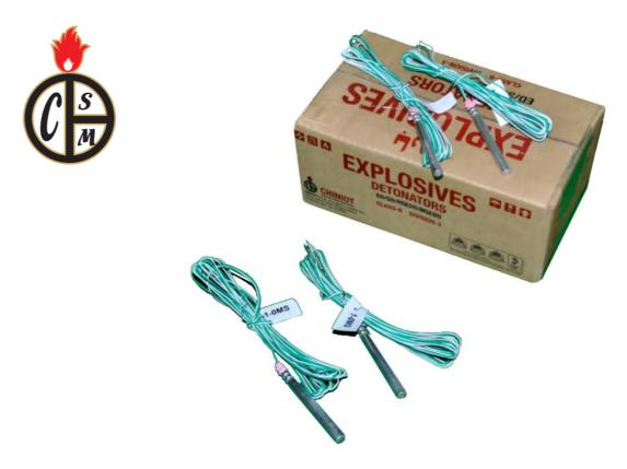
The usage of short delay detonators in blasting has been extensive. These detonators have a composition similar to electric or plain detonators, with the addition of a delay element positioned between the fuse head and primary charge. The delay element is activated by an electric impulse. Electric detonators with delays of milliseconds or half-seconds are commonly employed in activities such as quarrying, open pit operations, and breaching projects.
