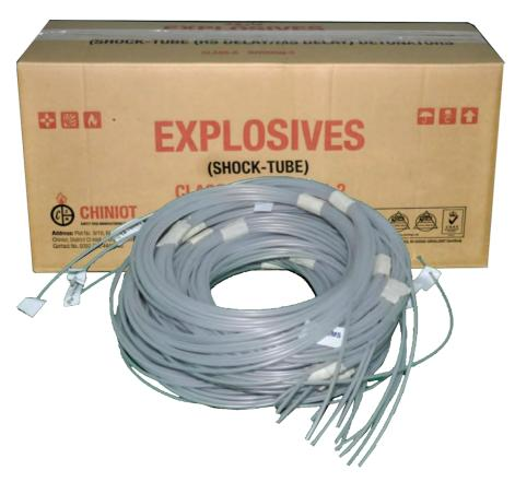
The signal shock tube consists of a narrow plastic tube coated inside surface with a very thin layer of high explosives. Shock tube can be initiated by detonators, detonating cord & mechanical shot shell starter device. In resulting shock ways travels at high speed (2000 m/s) through the tube towards detonator connected at the other end.
