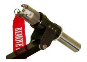
**Breech with safety pin.** Disruptor breech is upgraded from the older Pigstick version that it has a safety pin to keep the terminals short and cartridge is connected just when it has been deployed. This enables a bomb technician to set up the disruptor at the incident control point and spending minimum time at IED.
